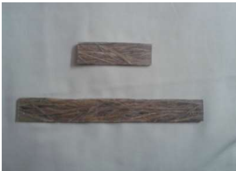
Fig 6.Specimen for tensile and impact test
