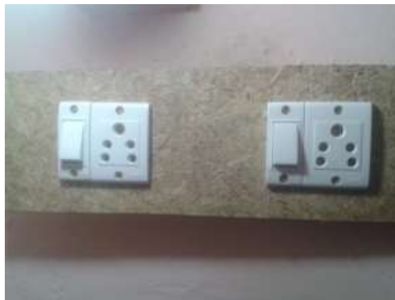
Fig 8. Composite plate as switch board
